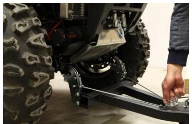
6. To adjust the angle of the blade, loosen the M10 x 35 bolts and turn the sides connector to a suitable position so that the height adjusters would be parallel to the ground.
