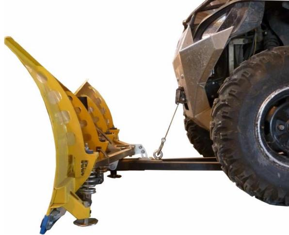
2. To change the plough's angle, remove/pull the pin up and turn the blade to the desired position.
