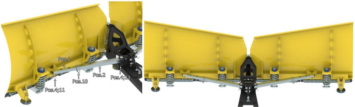
4. Install rubber cover 34.2007 between two sides of the plow. Use M6x16 bolts, Ø6 washers and M6 nylock nuts.
