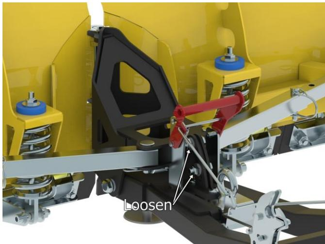
7. To adjust the working height of the blade, loosen the screw and set the skid at a suitable height. Push tube assembly should be parallel to the ground. Make sure that height adjuster is little bit lower than the blade. Plow should slide on height adjusters NOT on the blade!
